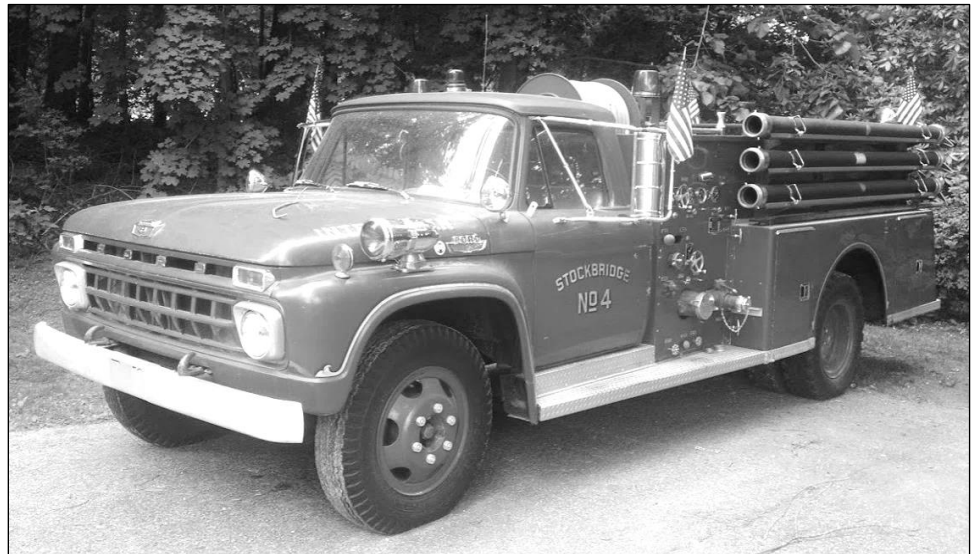
This 1965 Maxim 750 gpm pumper was built on a Ford commercial truck chassis. It served in Stockbridge, Massachusetts. It is an excellent example of the volunteer fire apparatus that served in many New England communities. It is owned by the Berkshire SPAAMFAA Chapter.
