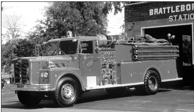
This 1970 Maxim S model pumper served in Brattleboro, Vermont. In 1989 it was rebuilt by Greenwood Emergency Vehicles of North Attleboro, Massachusetts.
