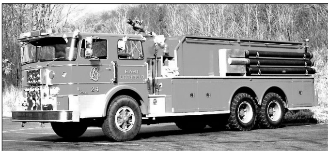
Farrar Fire Apparatus of Hopkinton, Massachusetts, built this pumper-tanker with a front mounted pump for Litchfield, Connecticut, in 1978 on a Duplex chassis.
