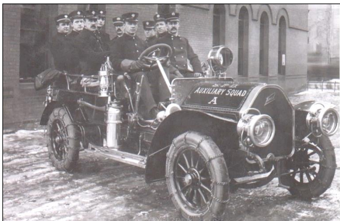
The fire department in Springfield, Massachusetts, was a pioneer in the adoption of motor fire apparatus. Among these was this squad wagon built by the Knox Automobile Company of Springfield.
